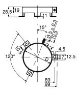
Fig. 4 - Dimensional outline of clamp for case Ø D = 76 mm
