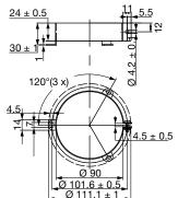
Fig. 5 - Dimensional outline of clamp for case  $\emptyset$  D = 90 mm
