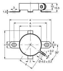
Fig. 9 - Dimensional outline of clamp for case Ø D = 25 mm, 30 mm and 40 mm
