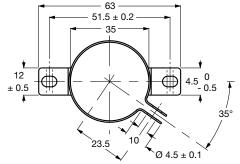
Fig. 10 - Dimensional outline of clamp for case Ø D = 35 mm
