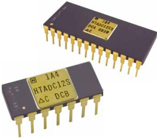
The HTADC12 is a high temperature, single supply, 12-bit, 100kSPS, analog-to-digital converter with on-chip buffered voltage reference and an on-chip analog input buffer. The HTADC12 uses a Successive Approximation Register (SAR) architecture that does not require an input sample-and-hold amplifier to provide 12-bit resolution at 100 kSPS data rates
