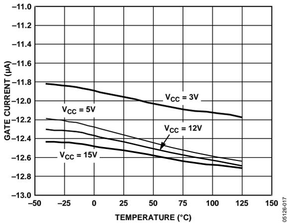
Figure 30. GATE Current (up) vs. Temperature
