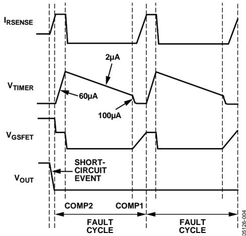
Figure 40. ADM1172-1 Automatic Retry During Overcurrent Fault
