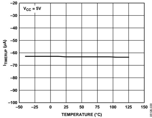
Figure 15.  $I_{TIMERUP}$  (During Cct Breaker Delay) vs. Temperature
