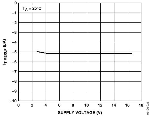
Figure 12.  $I_{TIMERUP}$  (In Initial Cycle) vs. Supply Voltage
