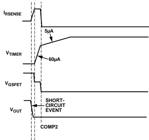
Figure 41. ADM1172-2 Latch Off After Overcurrent Fault
