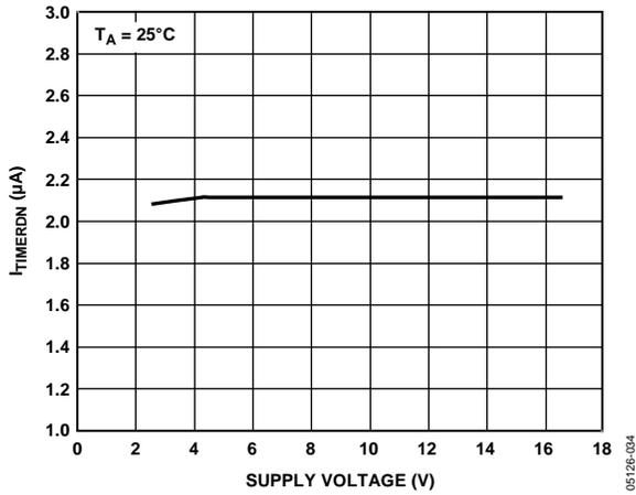
Figure 16.  $I_{TIMERDN}$  (In Cool-Off Cycle) vs. Supply Voltage
