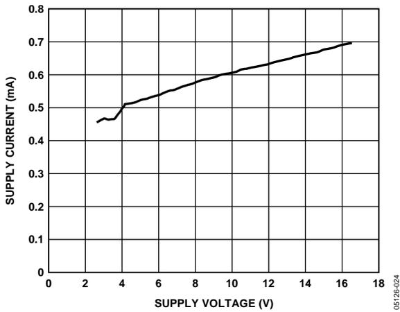
Figure 5. Supply Current vs. Supply Voltage (GATE On)
