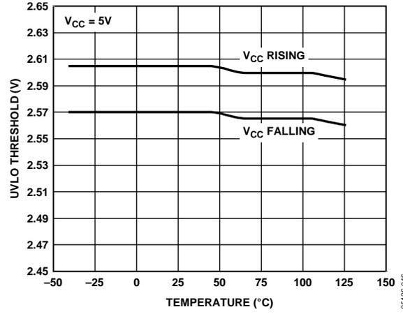
Figure 7. UVLO Threshold vs. Temperature
