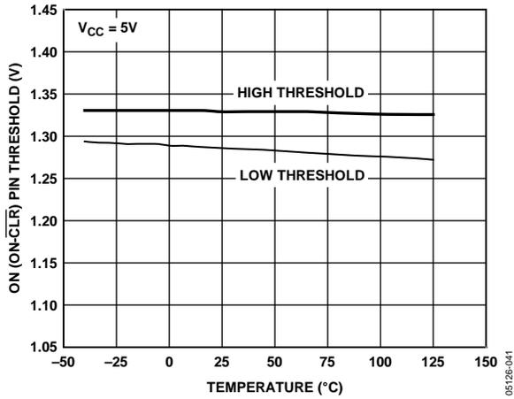
Figure 23. ON (ON-CLR) Pin Threshold vs. Temperature
