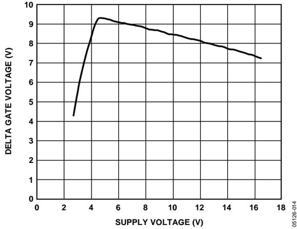
Figure 10. Delta GATE Voltage vs. Supply Voltage
