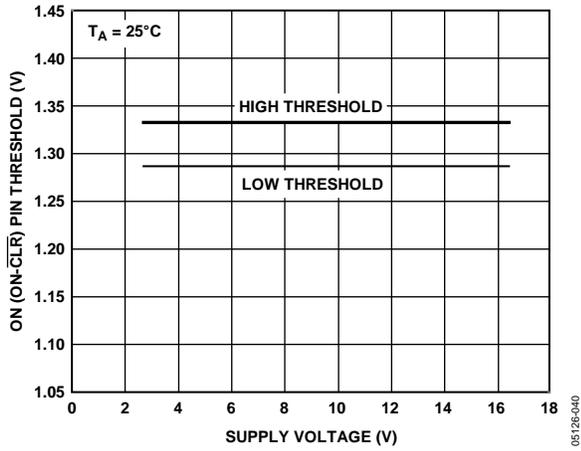
Figure 22. ON (ON-CLR) Pin Threshold vs. Supply Voltage
