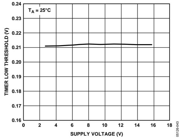
Figure 20. TIMER Low Threshold vs. Supply Voltage
