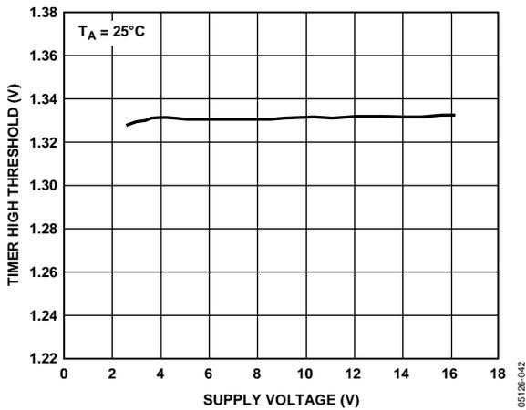
Figure 18. TIMER High Threshold vs. Supply Voltage
