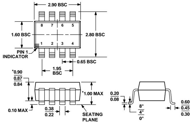
\*COMPLIANT TO JEDEC STANDARDS MO-193-BA WITH THE EXCEPTION OF PACKAGE HEIGHT AND THICKNESS.
