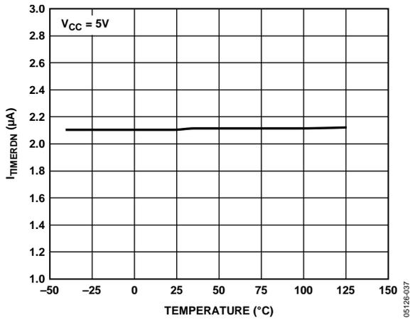
Figure 17.  $I_{TIMERDN}$  (In Cool-Off Cycle) vs. Temperature
