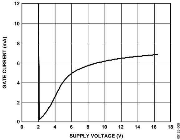
Figure 28. GATE Current (Down) vs. Supply Voltage
