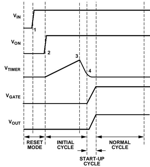
Figure 38. Power-Up Timing
