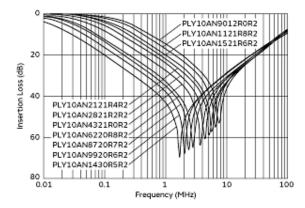
Differential Mode Insertion Loss (Typ.)
