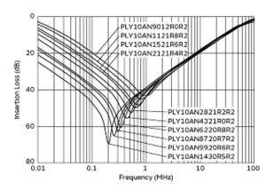
Common Mode Insertion Loss (Typ.)
