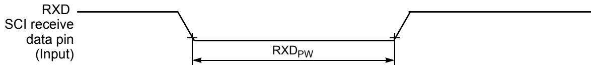
Figure 10-17 RXD Pulse Width
