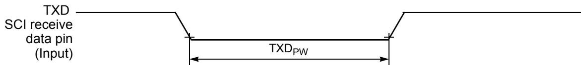
Figure 10-18 TXD Pulse Width
