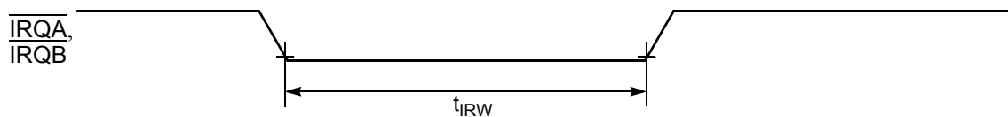
Figure 10-7 External Interrupt Timing (Negative Edge-Sensitive)
