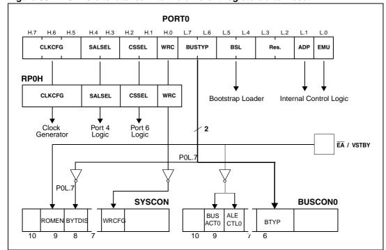
Figure 33. PORT0 bits latched into the different registers after reset
