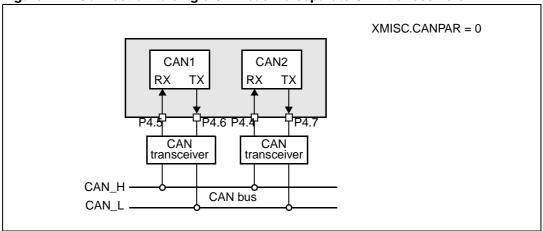
The ST10F273E also supports single CAN Bus multiple (dual) interfaces using the open drain option of the CANx\_TxD output as shown in *Figure 12*. Thanks to the OR-Wired Connection, only one transceiver is required. In this case the design of the application must take in account the wire length and the noise environment.
