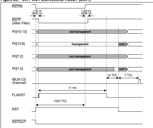
Figure 25. SW / WDT bidirectional RESET (EA=1)
