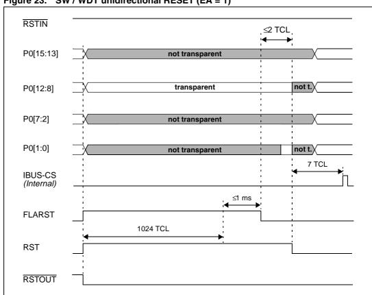
Figure 23. SW / WDT unidirectional RESET (EA = 1)
