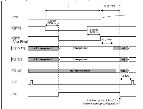
Figure 18. Asynchronous hardware RESET ( $\overline{EA} = 0$ )
