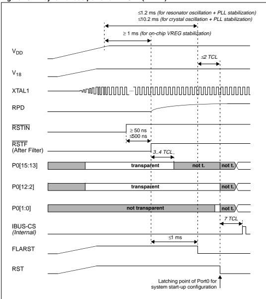
Figure 15. Asynchronous power-on RESET ( $\overline{EA} = 1$ )
