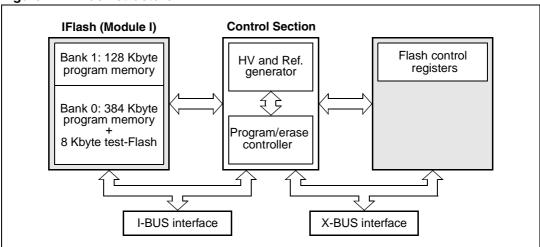
The programming operations of the flash are managed by an embedded Flash Program/Erase Controller (FPEC). The High Voltages needed for Program/Erase operations are internally generated.
