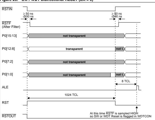
Figure 26. SW / WDT bidirectional RESET ( $\overline{EA} = 0$ )
