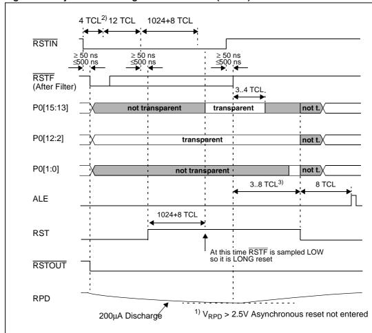
Figure 22. Synchronous long hardware RESET ( $\overline{EA} = 0$ )
