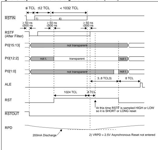
Figure 20. Synchronous short / long hardware RESET ( $\overline{EA} = 0$ )
