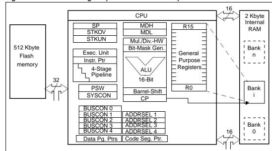
Figure 5. CPU block diagram (MAC unit not included)
