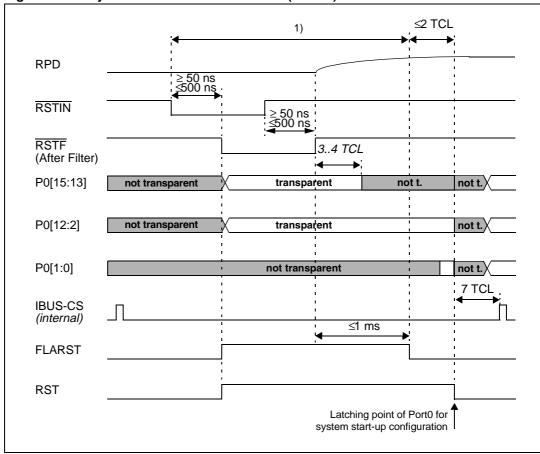
Figure 17. Asynchronous hardware RESET (EA = 1)
