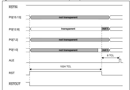
Figure 24. SW / WDT unidirectional RESET ( $\overline{EA} = 0$ )
