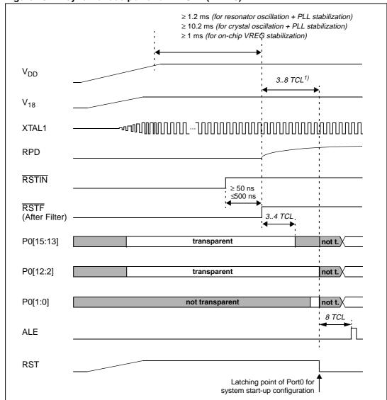
Figure 16. Asynchronous power-on RESET ( $\overline{EA} = 0$ )
