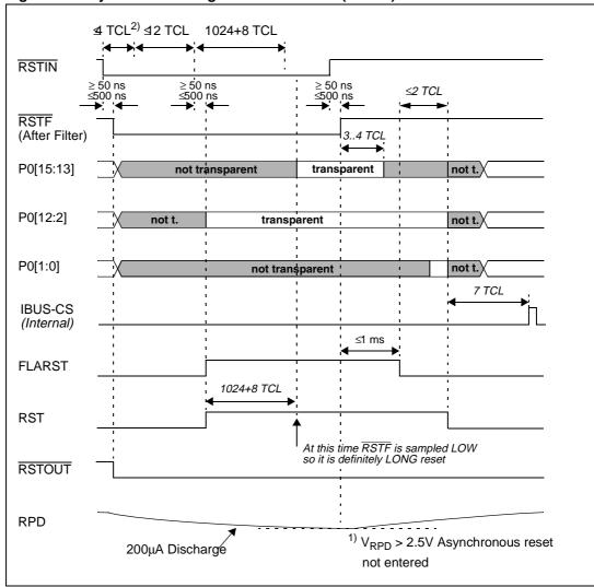
Figure 21. Synchronous long hardware RESET (EA = 1)
