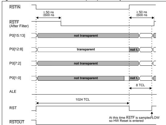
Figure 27. SW / WDT bidirectional RESET (EA=0) followed by a HW RESET
