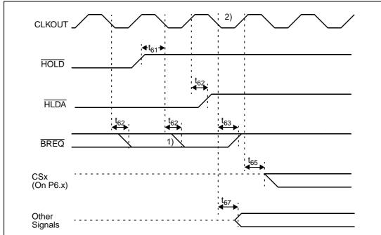
Figure 58. External bus arbitration (regaining the bus)
