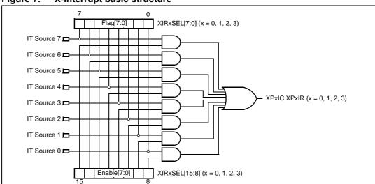
Figure 7. X-Interrupt basic structure
