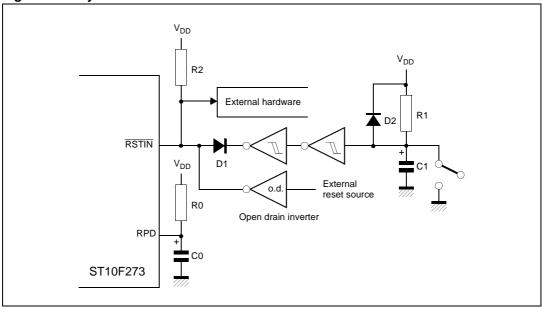
Figure 30. Internal (simplified) reset circuitry
