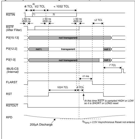
Figure 19. Synchronous short / long hardware RESET ( $\overline{EA} = 1$ )
