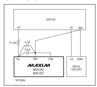
Figure 11. Power-Supply and Grounding Connections
