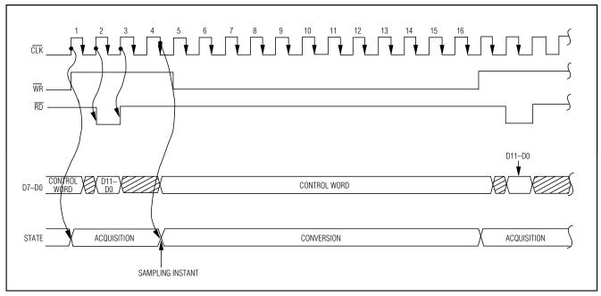
Figure 10. Timing Diagram for Fastest Conversion
