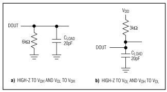
Figure 1. Load Circuits for Enable/Disable Times
