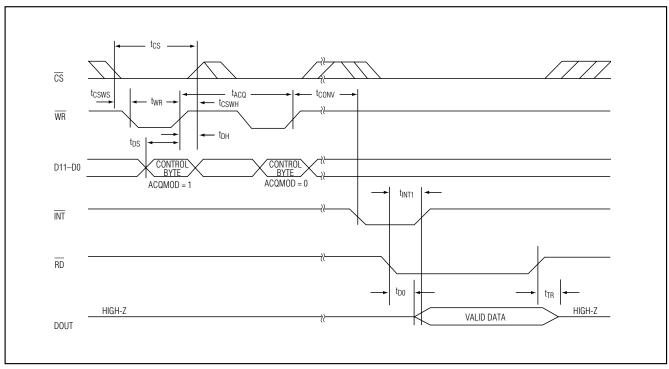
Figure 5. Conversion Timing Using External Acquisition Mode
