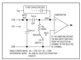
Figure 3b. MAX1267 Simplified Input Structure
