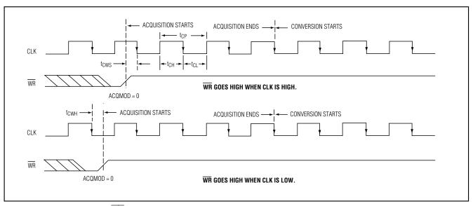
Figure 6a. External Clock and WR Timing (Internal Acquisition Mode)
