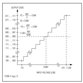
Figure 9. Bipolar Transfer Function
