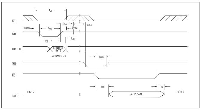
Figure 4. Conversion Timing Using Internal Acquisition Mode
