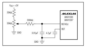
Figure 7. Reference Adjustment with External Potentiometer
