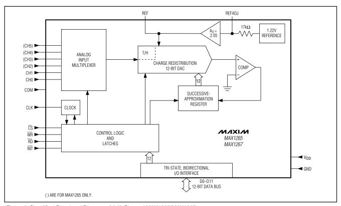
Figure 2. Simplified Functional Diagram of 6-/2-Channel MAX1265/MAX1267
