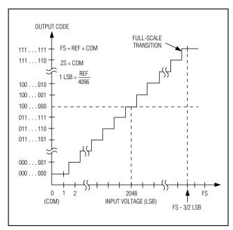
Figure 8. Unipolar Transfer Function
