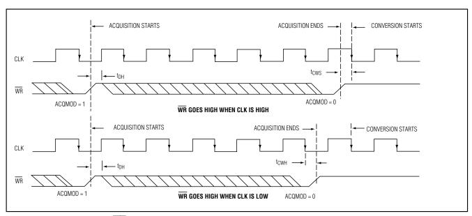
Figure 6b. External Clock and WR Timing (External Acquisition Mode)
