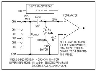
Figure 3a. MAX1265 Simplified Input Structure
